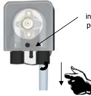
Step 14 Screw the cap with the PE tubing (white) onto the pump.
